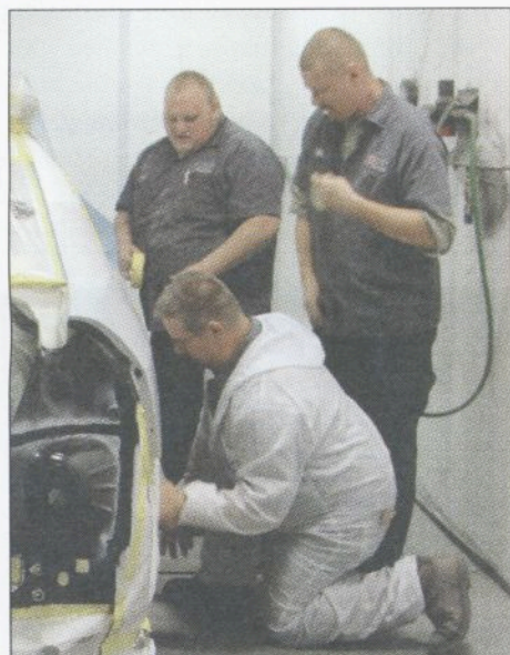
Members of the Zara's Collision Center team mask off a vehicle in the shop's paint booth. This booth was recently retrofitted with an air movement system purchased from MJF Equipment Sales to accommodate the use of Sikkens AutoWave waterborne paint.
